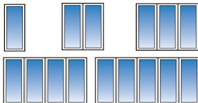
Multiple casement windows are available in a continuous mainframe with two, three, four or five-lite configurations. Virtually any combination of fixed-lites, with hinged-left or hinged-right operating casement windows are available.
